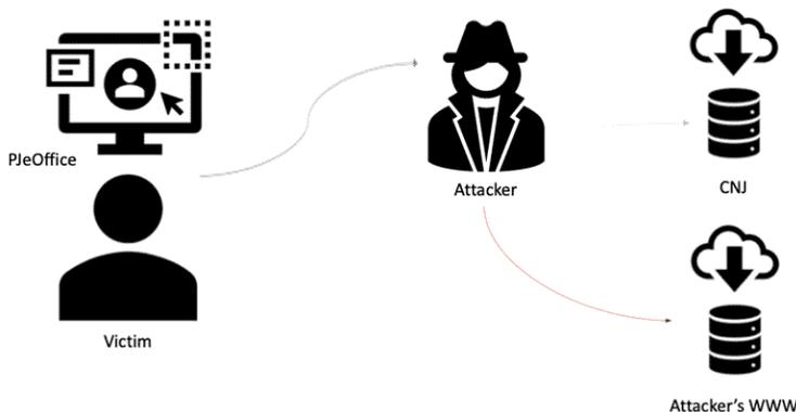
CNJ PJe's platform does not properly validate the integrity and authenticity of the update prior to installation. As such, the attacker is able to force the installation of a forged application on the device of the vulnerable user. [figure 3]
