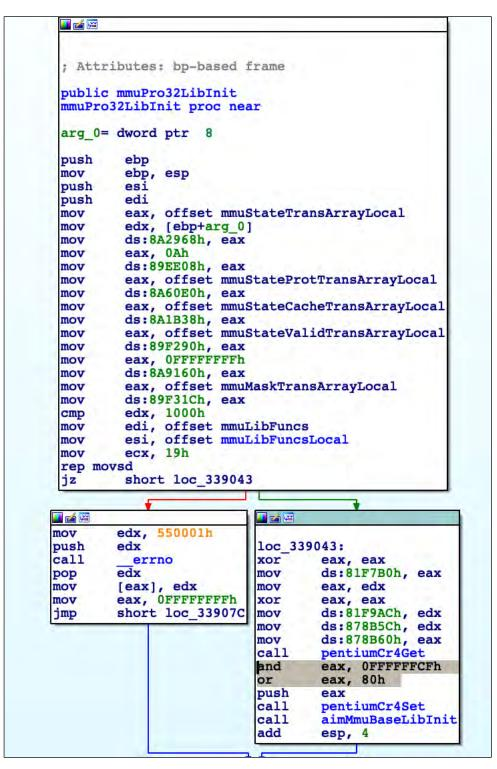
Figure 28. MMU Initialization Routine in CIS/MS VxWorks
