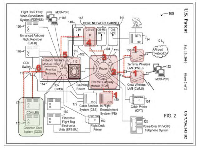
Figure 12. Basic Attack Surface
