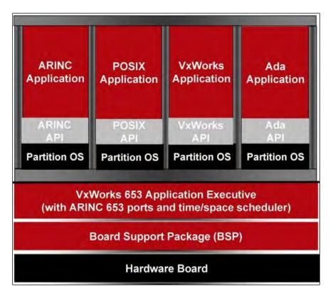
Figure 1. VxWorks 653 Architecture<sup>12</sup>
