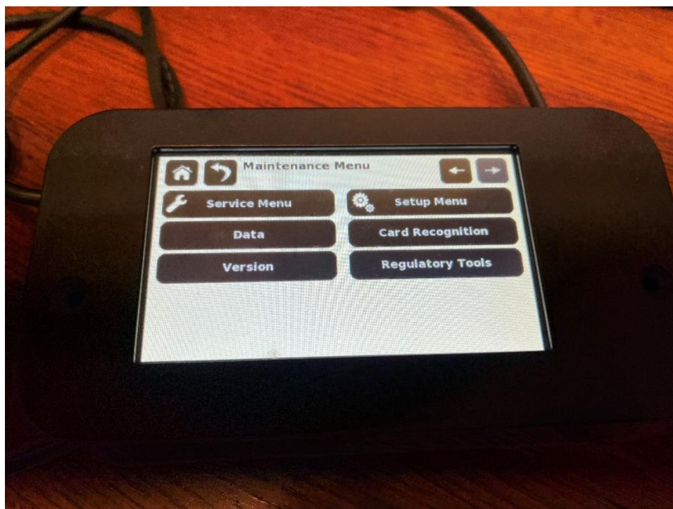
Figure 40. DM2 External Display Module Maintenance Menu via X11 forwarding
