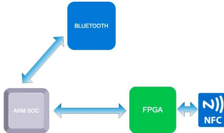
The Proxmark project provides certain APIs for communication with the Bluetooth chip and FPGA, which we'll use during the programming phase. Third-party standalone modules like `hf_reblay` can help to more quickly understand how this communication works.
