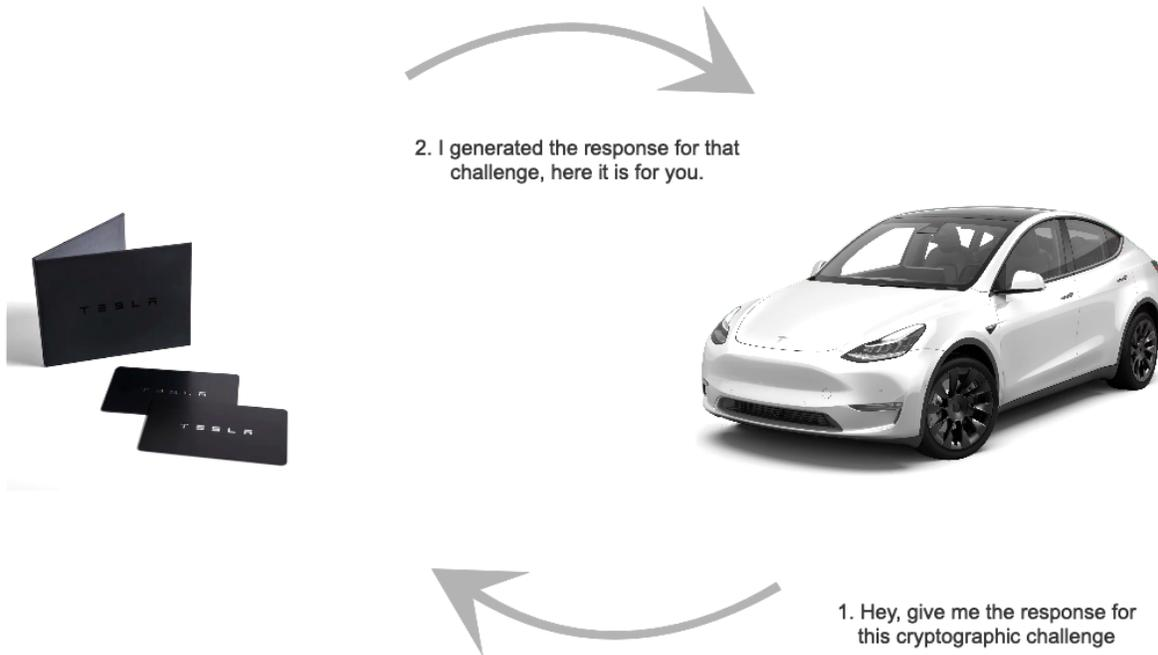
To better understand what's going on between the vehicle and the NFC card, we must reverse-engineer the protocol. For this attack, IOActive used the Proxmark RDV4.0 device to sniff these communications. The next image is the result, illustrating the NFC communication that takes place while opening the vehicle with the NFC card. The packets outlined in blue are the low-level NFC communications, and those outlined in red are the application layer (APDUs):
